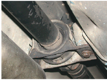
Figure 5.90 This rubber mounted bearing prevents propshaft whip
